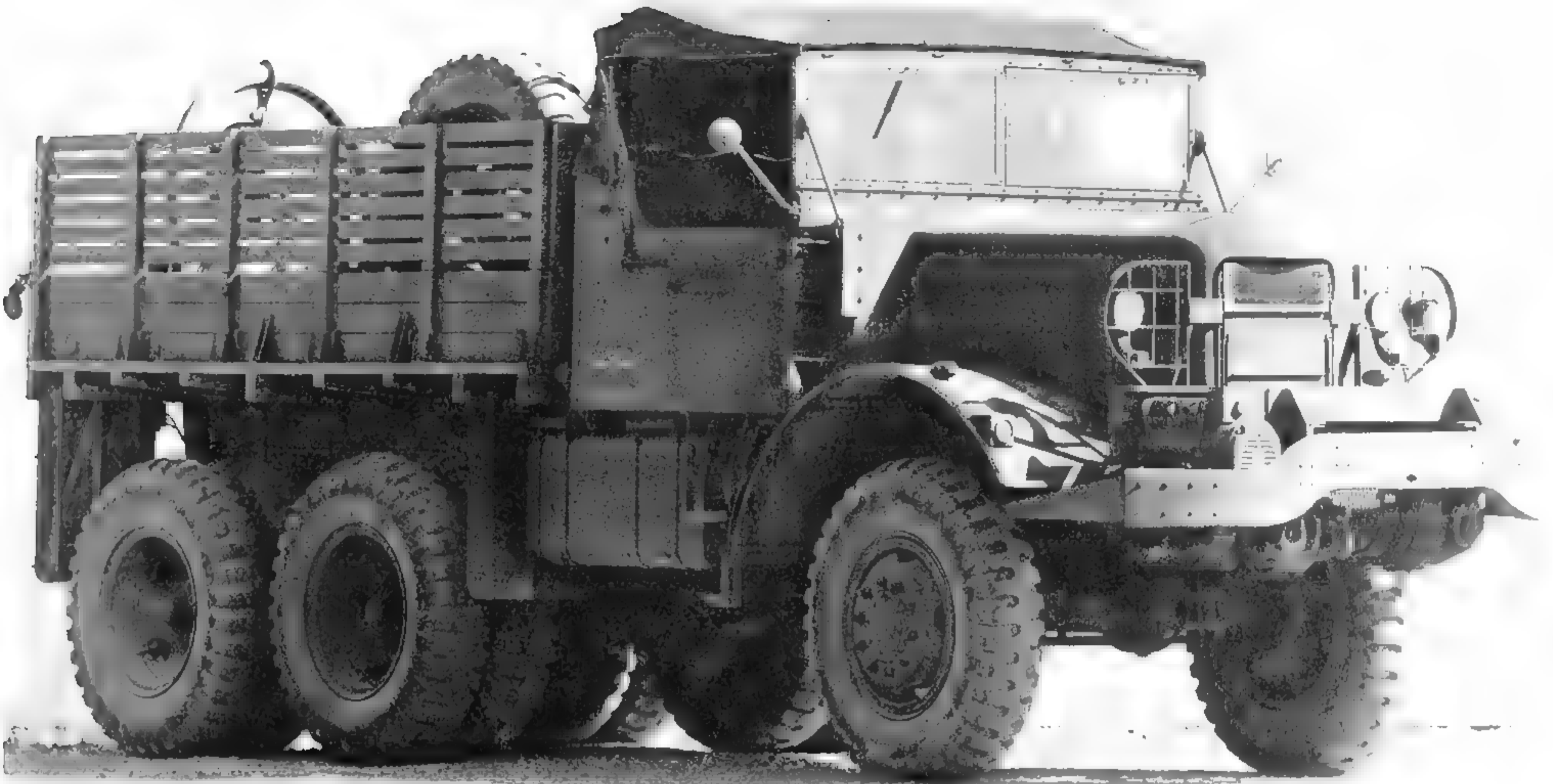
The NO-6, like the other production NOs, had the traditional military troop seat and side board arrangement. The lower section of the side boards aft of the spares hinged down to provide seating. The rear-mounted derrick is barely visible in this 1944 Studebaker Proving Ground photo. (U.S. Army photo)
